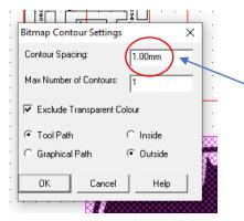
9. A Bitmap contour spacing pop up will appear. This basically traces the image. *Change the contour* from 5.00mm to *1.00mm*.
