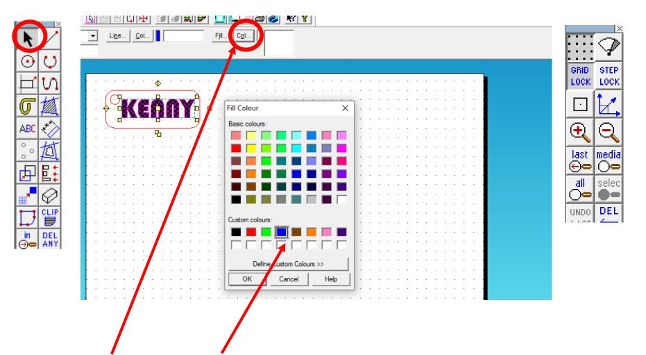
19. Whilst your name is highlighted Click on the fill *Col* tool shown to bring up the fill *colour palette* shown. Click on *blue* as this is to *engrave* on the laser cutter.
