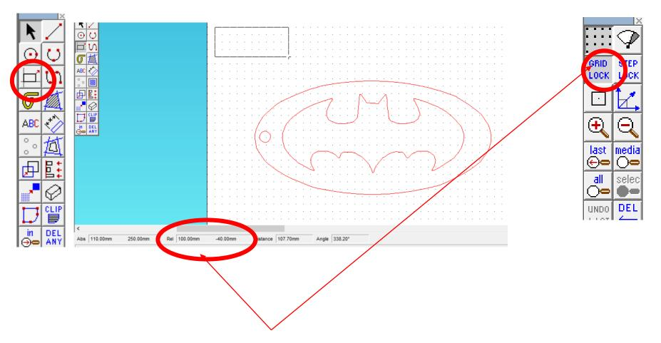
Select the *rectangle tool* shown. Draw a square the measures *100mm x 40mm*. You have to look at the *Rel tool box* shown at the bottom of the screen to size it correctly.
