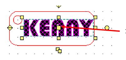
18. Using the *select tool* move it using the centre square shown on to your key ring. Position and resize
