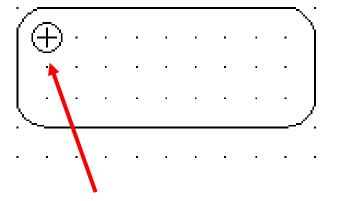
Position the *circle* shown on the key ring. This is the hole for the keyring and has a 1cm diameter
